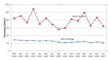
The performance graphs (left) compares (i) 4.7 m long GEE *Earthing* and (ii) 4.7 m long GI strip *Earthing* (i.e. bare conductor buried in soil).
