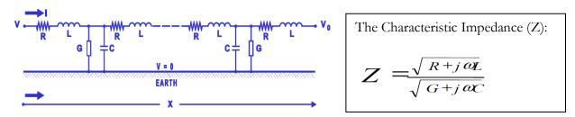
Where: R = Resistance, L = Inductance, C = Capacitance, G = Conductance  $\omega$  = Angular frequency (2 $\pi$ f), j = imaginary unit
